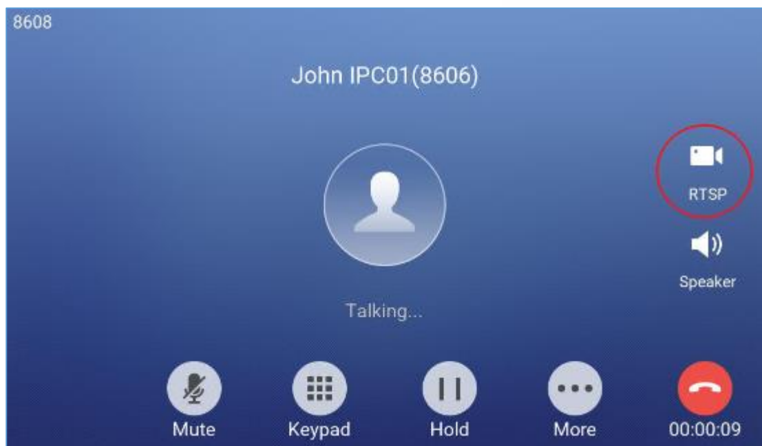
Figure 18: GSC3570 Switching to RTSP stream during an active SIP call
