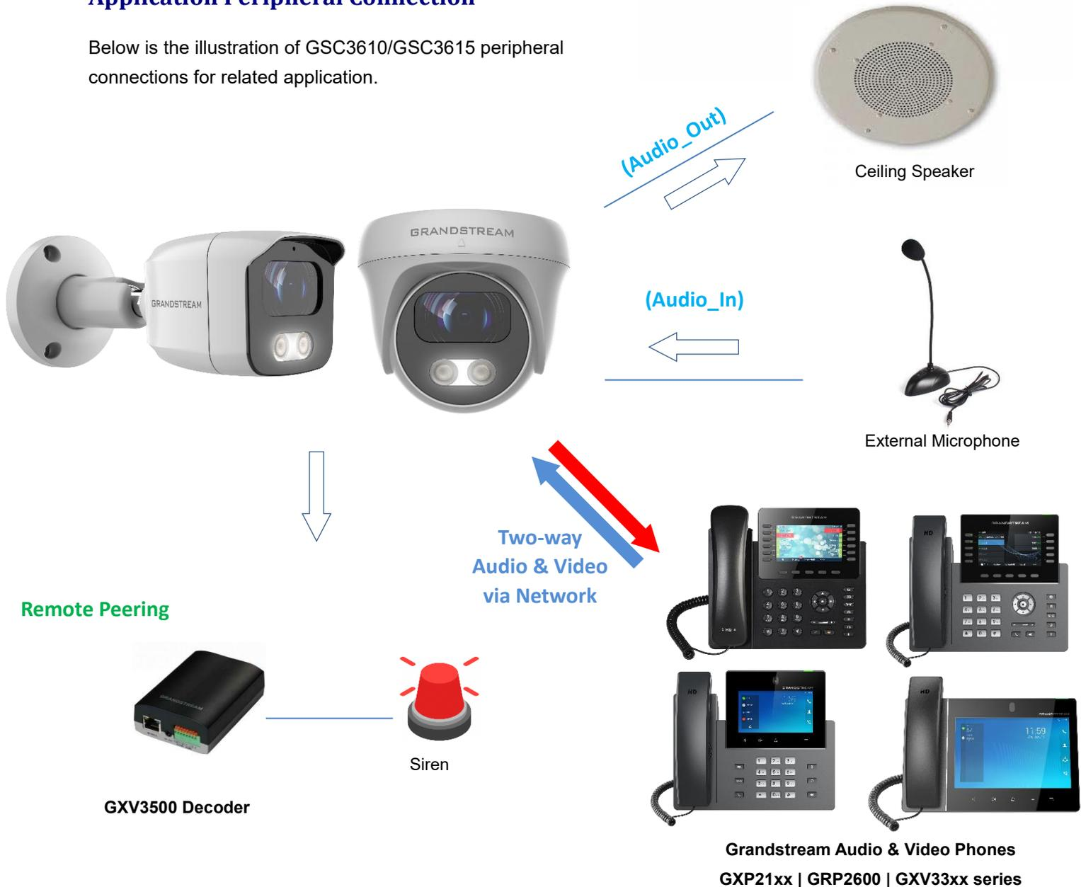
Figure 7: Application Peripheral Connection for GSC3610/GSC3615
