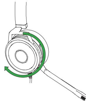
The GU3005 can be worn on the left or right by flipping the microphone to the other side (235° limit).
