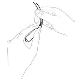
To avoid low or distorted sound, and to provide clear and crisp telephone calls, the microphone should be positioned within 0.5 inches of your mouth. The microphone boom arm will move in a variety of directions to ensure the best fit.
