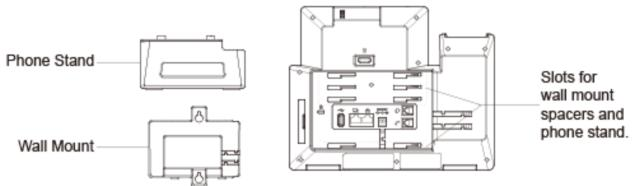
Figure 4: Phone Stand and Mounting Slots on GXV3350
