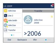
To cancel the transfer you can either press the **Cancel**softkey on the display screen, press \_\_\_\_, or hang up the handset.
