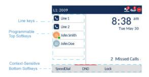
The state-sensitive softkeys change depending on the state of the phone and are used to perform different functions when the phone is in an idle, connected, outgoing, or busy state.
