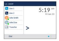
This screen displays the Dial key at the bottom. This key is context-sensitive and cannot be changed.
