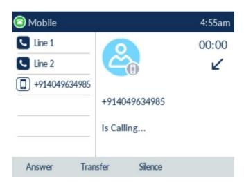
To answer the incoming mobile call using your Mitel 6920w IP phone, lift the handset for handset operation, or press the (Speaker/Headset) key, tap the blinking (Bluetooth Line key, or tap the Answer softkey for handsfree operation.
