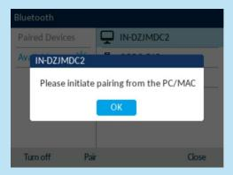
After your PC is paired with the 6920w IP Phone, the PC device appears in the list of paired devices on the Mitel 6920w IP Phone and the device automatically connects with the IP Phone once paired. If a mobile phone is already connected, the IP Phone displays a message **Do you want to connect to this device?**
