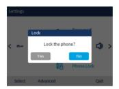
3. At the Lock the phone? prompt, navigate to the Yes button and press the select button. The message Phone is locked and lock icon displays on the Home screen. Additionally the Message Waiting Indicator (MWI) will turn on.
