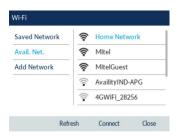
**3.** Select an SSID (that is, the name of a Wi-Fi network; for example, Home Network) from **Available Networks** press **Connect** softkey. If the SSID is secured, a password prompt appears.
