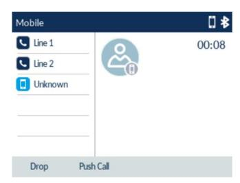
Tap the Mobile Line key to pull the mobile call audio from your mobile phone to the Mitel 6920w IP Phone.
