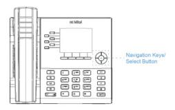
There are four directional keys (up, down, left, and right) on the navigation cluster that can be used to navigate through the various applications and settings menus. The center key acts as a **Select** button that is used to set options and perform actions such as dialing out from the **Contacts** or **Call History** applications.
