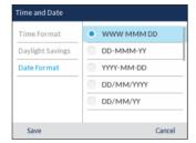
9. With **Date Format** highlighted press the right navigation key to move to selection column.
