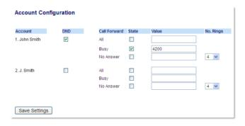
**5.** For each account, enable DND by placing a check mark in the box. Disable DND by unchecking the box.
