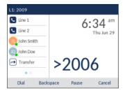
With the phone in an idle state and on-hook, simply use the dialpad to enter the number you wish to call, and after reviewing the number, press the **Dial** softkey. Use the **Backspace** softkey to correct any errors and the **Pause** softkey to insert pauses.
