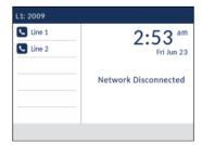
Check that the cables are tightly connected to the phone and to the wall jack. The phone should automatically detect when it is reconnected and remove the Network Disconnected prompt from the screen. However, if changes have been made to your phone's network settings, you may need to restart your phone. Check with your System or Network Administrator for assistance.
