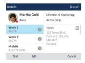
**4.** Press the Dial softkey, select button, Line button, button, or pick up the handset to dial the contact's phone number.
