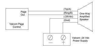
Refer to Figure 1 for audio and electrical connections. Category 3 24 AWG structured cable may be used for all connections.
