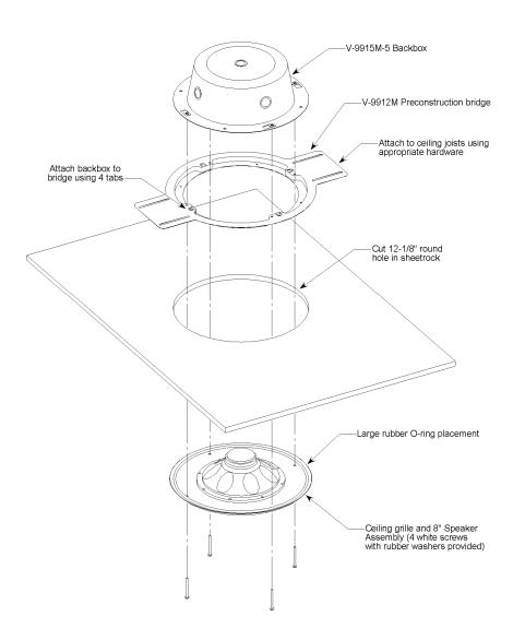
FIGURE 3: V-1040 INSTALLATION INSTRUCTIONS HARD CEILING
