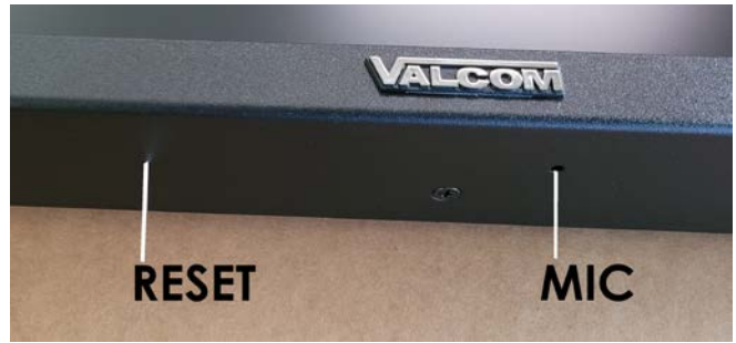
Figure 2. Reset and Microphone Location
