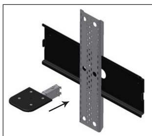
Lock in PS-CTR to Central Support using tabs. Adjust the length of the PS-CTR and tighten Buttonhead Bolt.
