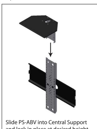
Slide PS-ABV into Central Support and lock in place at desired height using tabs.
