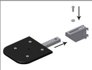
Using the Buttonhead Bolt 1/4 x 3/4", bolt the Center Extension with Acrylic to the Center Arm.
