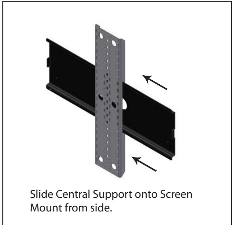
Slide Central Support onto Screen Mount from side.
