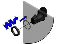
Slide and twist the Lock Washer and Nut (R), respectively, onto Cylinder (U) as shown in diagram. Ensure that it's placed in the correct position as shown in the diagram.
