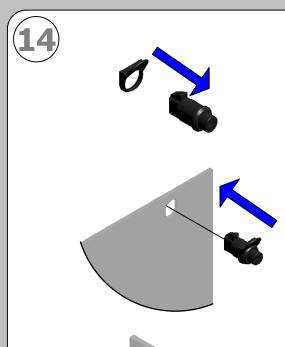
Slide Pull (T) over Cylinder (U). The Flange must be as shown in the diagram
