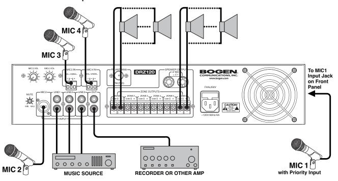
Note: Individual zone output levels are set by adjusting the Zone Volume Controls on the Front Panel.
