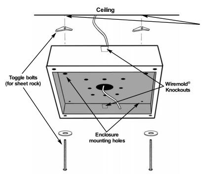
Use two of the enclosure's mounting holes as a template (diagonally opposed), and mark screw hole locations. If toggle bolts will be used, drill two, 1/2" diameter holes in the mounting surface, otherwise drill a hole appropriate for hardware being used.
