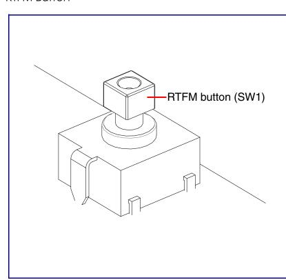
When the device is operational and linked to a network, you can use the Reset Test Function Management (RTFM) button (SW1 [see picture]) to announce the device's IP address or restore the device to the factory default settings.
