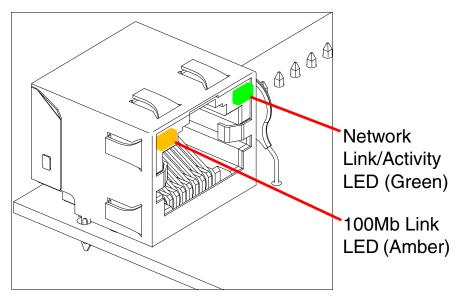
3.2. The green **Network Link/Activity** LED blinks off once during the boot up process when the device begins DHCP addressing and autoprovisioning attempts, and then comes on again and remains constant (solid green). The amber **100Mb Link** LED may be blinking depending on the network activity.
