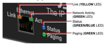
3.2. The GREEN/BLUE Status LED will blink during the boot process. The GREEN Paging LED will illuminate solid during initial network setup and then turns off. After the initialization process the GREEN/BLUE Status LED will blink twice a second.
