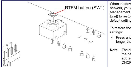
When the device is operational and linked to a network, you can use the Reset Test Function Management (RTFM) button (SW1 [see picture]) to restore the device to the factory default settings.
