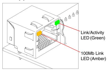
3.2. The Green **Link/Activity** LED blinks off once during the boot up process and then comes on again and remains constant (solid green). The amber **100Mb Link** LED may be blinking depending on the network activity.
