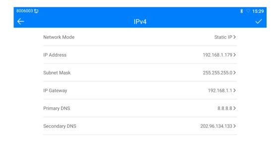
Picture 102 - Static IP network mode
