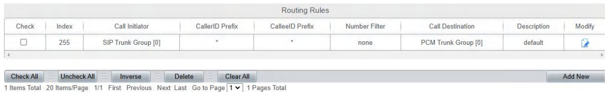
Figure 3-25 IP→PSTN Routing Rule Configuration Interface
