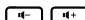
In idle mode or during ringing: increase or decrease ringer volume In communication: increase or decrease handset or hands-free volume
