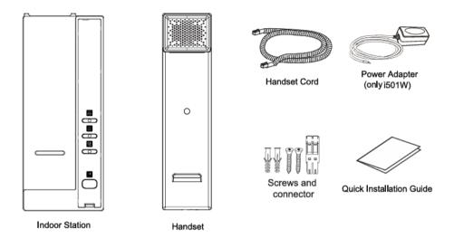
**Note**: The i501W comes with a standard power adapter, while the i501 supports PoE for both network connectivity and power supply.
