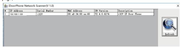
The above picture shows the device information founded by the IP scanning tool, and the IP address is dynamic.
