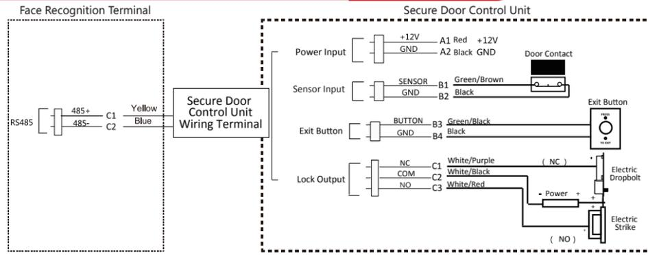
The secure door control unit should connect to an external power supply separately. The suggested external power supply is 12 V, 0.5 A.
