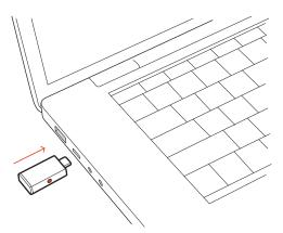
2 Connection is successful when you hear "PC connected" and the USB adapter turns solid. NOTE Adapter design may vary.
