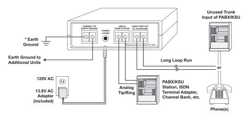
\* **Note:** To increase surge protection, and to give the long loop run an earth ground reference, fasten a wire from the screw terminal to Earth Ground (grounding rod, water pipe, etc.).
