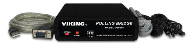
The **PB-100** is used to provide status polling of Viking **1600A** Series Emergency Phones or remote programming of **AES-2000** Entry Systems. The **PB-100** can connect to an unused serial port on your PC or use the included RS-232 to USB converter cable to connected to a USB port. Downloadable software is available with these two applications along with software for programming other Viking products.
