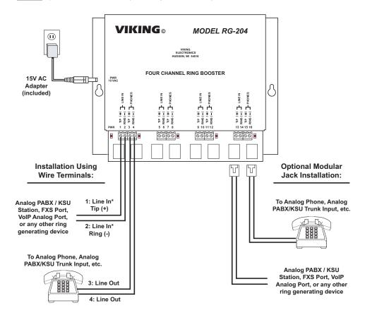
\* IMPORTANT: "LINE IN" is polarity sensitive. If wired in reverse polarity, the RG-204 may trip ringing after the first ring.
