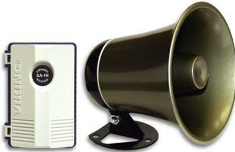
The Viking model **SA-1H** is a 5 inch paging horn that includes a 1.5 watt power amplifier, an infrared remote control detector, and an integrated digital volume control. The **SA-1H** self amplified paging horn uses a proprietary two wire protocol in which both 40 volts DC power and audio are combined on the same pair of wires. It is designed for direct connection to the Viking Model **SA-25** Self Amplified Paging Control unit, or use the Viking model **SA-X12**
