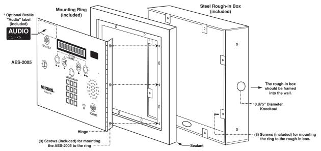
Important: If the enclosure is to be mounted outdoors, use an appropriate sealant around the outer edge of the mounting ring.
