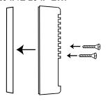
Attach the cover to the base with the two included screws as shown.
