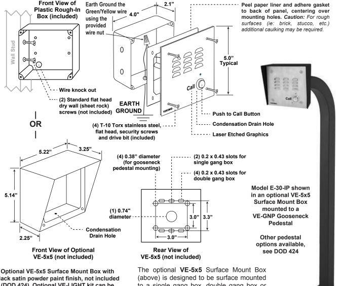
black satin powder paint finish, not included (DOD 424). Optional VE-LIGHT kit can be used to illuminate the faceplate when used with a VE-5x5 (DOD 428). WARNING: Do NOT use a wet location box. The optional **VE-5x5** Surface Mount Box (above) is designed to be surface mounted to a single gang box, double gang box or **VE-GNP** Gooseneck Pedestal (shown right). For more information on the VE-5x5 and VE-GNP, see DOD 424.
