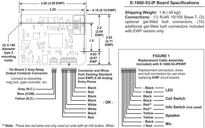
installing on a single button unit, cut off these two red wires and discard.
