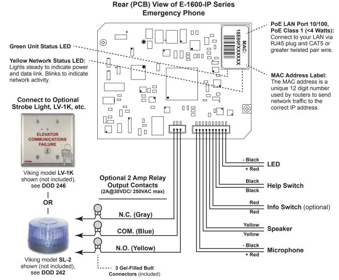
**Note:** The gel-filled (water-tight) butt connectors are designed for insulation displacement on 19-26 gauge wire with a maximum insulation of 0.082 inches. Cut off stripped wire ends before terminating.
