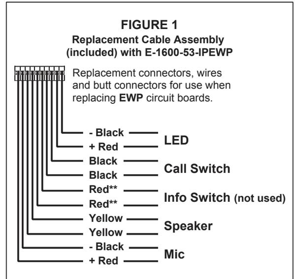
**\*\* Note:** These two red wires are only used on units with an Info button. When installing on a single button unit, cut off these two red wires and discard.
