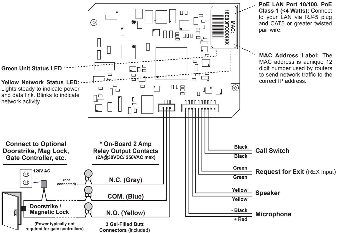
**Note:** The gel-filled (water-tight) butt connectors are designed for insulation displacement on 19-26 gauge wire with a maximum insulation of 0.082 inches. Cut off stripped wire ends before terminating.
