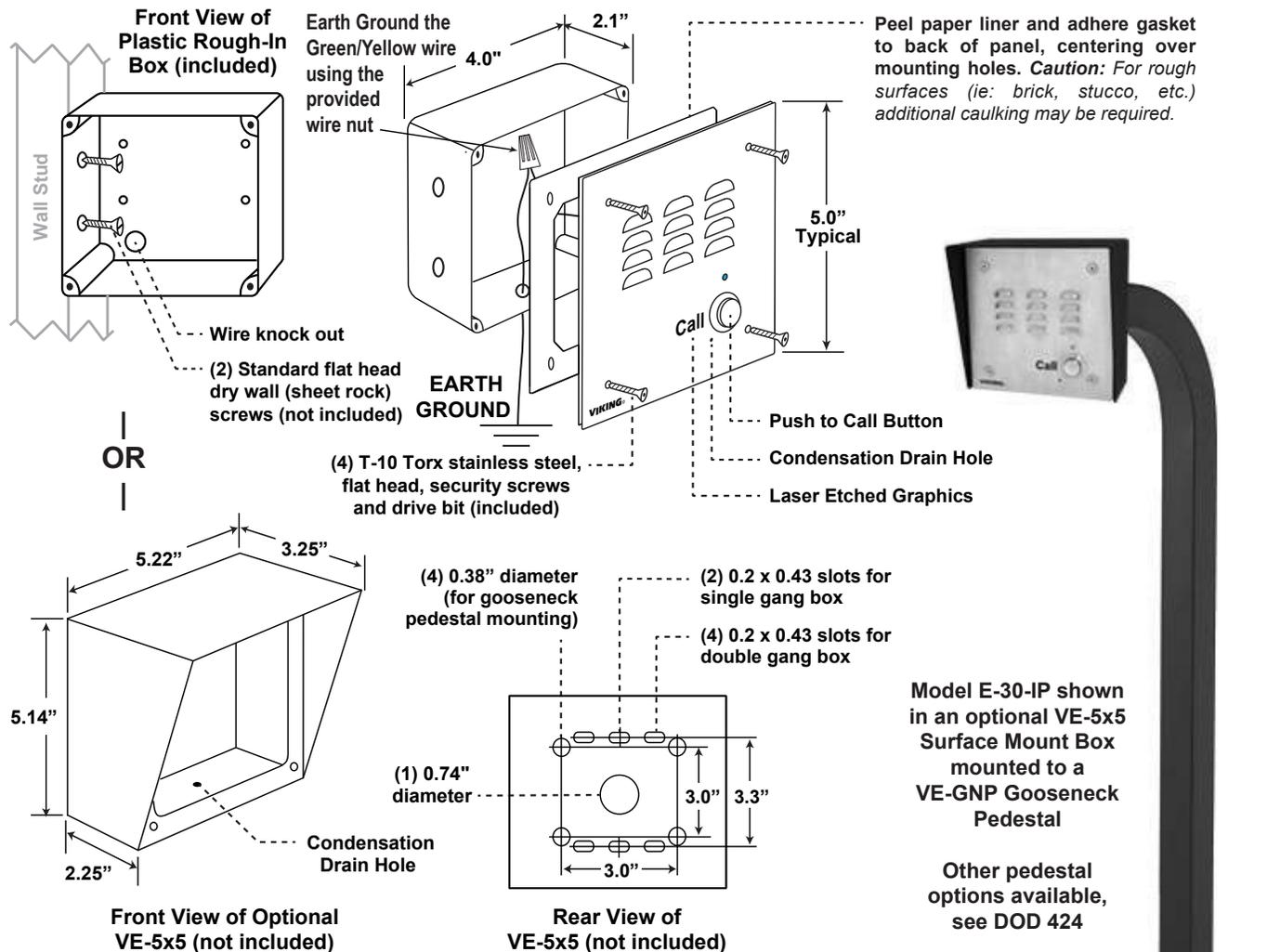
Optional **VE-5x5** Surface Mount Box with black satin powder paint finish, not included (DOD 424). Optional **VE-LIGHT** kit can be used to illuminate the faceplate when used with a **VE-5x5** (DOD 428).
