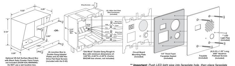
\* CAUTION: Excessive wire length and/or using a rough-in box with inadequate depth can apply force to the circuit board causing physical damage.
