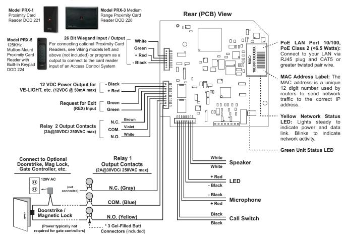
**Note:** The gel-filled (water-tight) butt connectors are designed for insulation displacement on 19-26 gauge wire with a maximum insulation of 0.082 inches. Cut off stripped wire ends before terminating.
