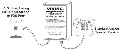
\* An FXS port lets you connect an analog telephone or device to an IP network.
