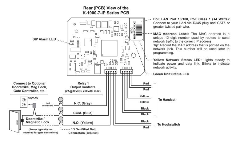
**Note:** The gel-filled (water-tight) butt connectors are designed for insulation displacement on 19-26 gauge wire with a maximum insulation of 0.082 inches. Cut off stripped wire ends before terminating.
