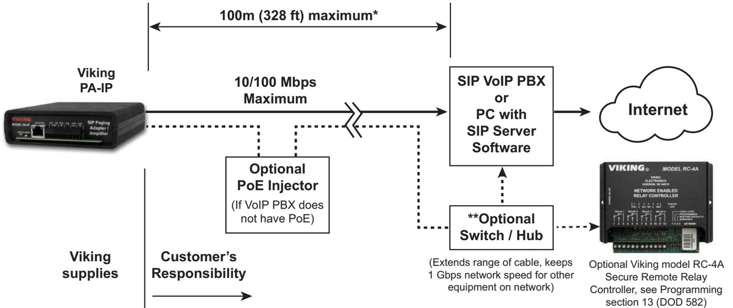
\* **Note:** A PoE extender can be used for an additional 100 meters per extender. For longer runs (up to 2 km / 1.2 miles) an ethernet to fiber media converter can be used.
