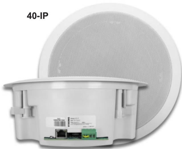
The Viking model **40-IP** Ceiling/Wall Speaker enables SIP endpoint paging and also allows for standard paging and background music via multicast. The speaker easily connects with a single CAT5/6 cable from your PoE switch. Its shallow depth allows the speaker to be conveniently mounted in a standard 2" x 4" stud wall or ceiling.
