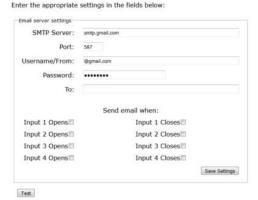
This page is for setting up email notification of input events. The **RC-4A** can be programmed to send an email if one of the inputs closes, and also if it opens. As described in **Programming A. Settings, 2. Input Status Phrasing**, the input status can be described as something other than "open" or "closed", and this customized description is used in the email.
