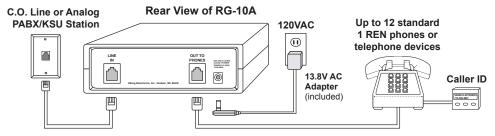
**Note:** In the event of a power outage, inbound and outbound calls are possible, although only phones installed ahead of the **RG-10A** will ring.
