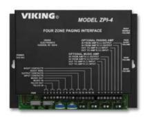
The **ZPI-4** is compatible with ringing analog PABX/KSU station ports (disconnects on silence, CPC, busy, Touch Tone "#" or time-out) as well as unused trunk inputs, and will interface directly with standard paging ports.
