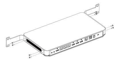
2. Push the MeetingEye 500 into the rack, and then fix it to the rack with screws.
