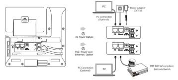
Note: The IP phone should be used with Yealink original power adapter (5V/1.2A)only. The use of the third-party power adapter may cause the damage to the phone. If you are connecting a PC to your phone, we recommend that you use the Ethernet cable provided by Yealink. If inline power (PoE) is provided, you don't need to connect the power adapter. Make sure the hub/switch is PoE-compliant.
