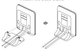
Align the snap-fits with the corresponding holes and push forward, snapping them into the holes.
